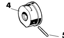
2) **No Drill Nut:** Tighten the nut (4) onto the shaft. Align the groves in the base of the nut with the groves in the central hub, so as to obtain two complete holes allowing insertion of the pins (5). Insert the pins, as shown in the drawing below, so as not to interfere with the inserting of the central cone gear
